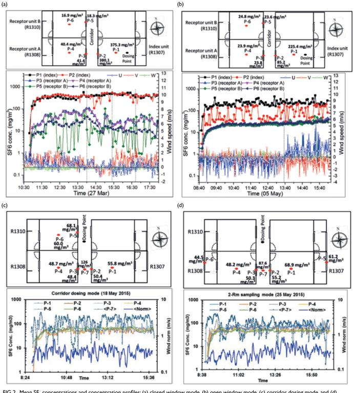
FIG 2. Mean SF<sub>6</sub> concentrations and concentration profiles: (a) closed window mode, (b) open window mode, (c) corridor dosing mode, and (d) 2-room mode
